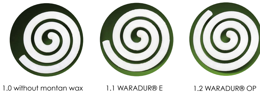
Figure 2: Flow spirals from PA compounds without flow aids and with WARADUR® E and WARADUR® OP
