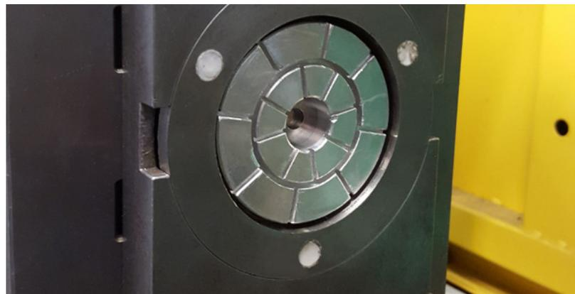
Figure 2: Tool cavity with core setter
