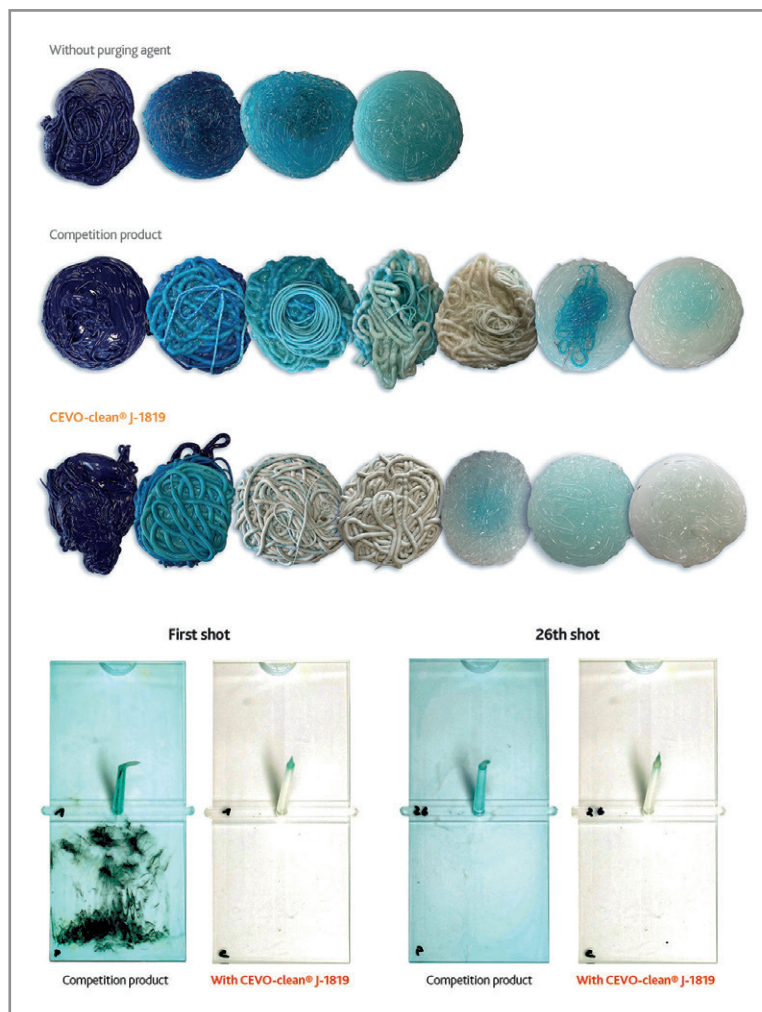
Trials carried out at Germany's Kunststoff-Zentrum Leipzig compared performance of Völpker's Cevo-clean J-1819 against a commercially-available competitor in a coloured transparent PMMA application. Figure 1 (upper image) compares the two purging compounds against cleaning with no purging agent; Figure 2 (lower image) shows injection moulded plaques produced on the first and 26th shots after the two purging compound cleans
