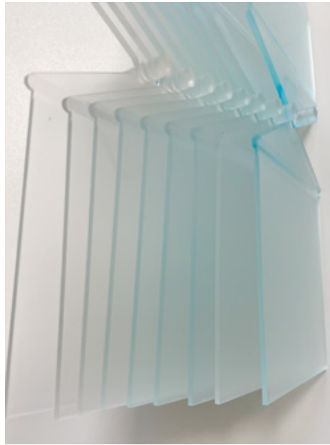
Fig. 3 Fast color change by using CEVO®-clean 1823/PMMA (1:4). See also Tab. 1.
