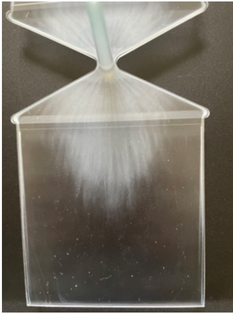
Fig. 2 Competitor: Streaks of the cleaning agent on the plates – even after rinsing with PMMA.
