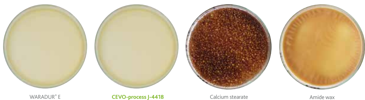
Figure 4: Colour stability under thermal stress (Laboratory Air Circulation Oven Heraeus UT 6120: 250 °C/30 min; Ca-stearate: 10 min)
