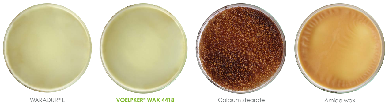
Fig. 4: Colour stability under thermal stress (Laboratory Air Circulation Oven Heraeus UT 6120: 250 °C/30 min; Ca-stearate: 10 min)
