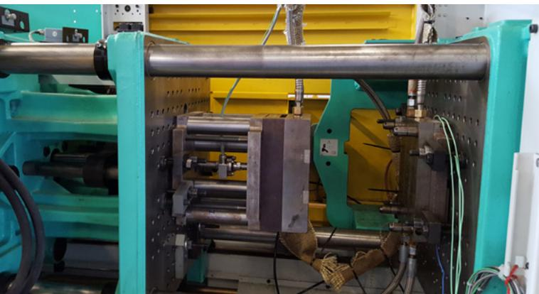
Figure 1: Clamping unit for the injection mould system / Integrated load cell (from left to right)
