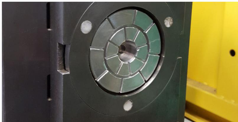
Figure 2: Tool cavity with core setter
