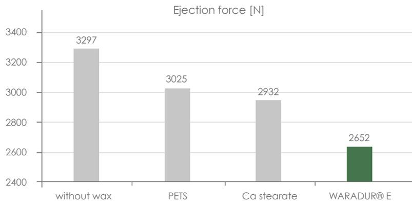
Figure 3: Ejection forces for the formulas tested
